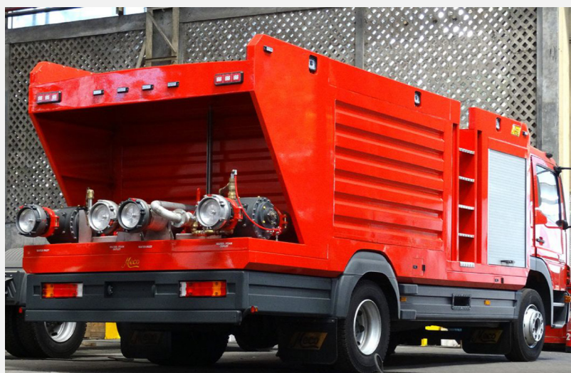
Foam truck for PERTAMINA oil company in Indonesia with 2 units FIREMIKS 8000-3-GP-F giving total capacity of 16.000 lpm and 3% dosing rate.
