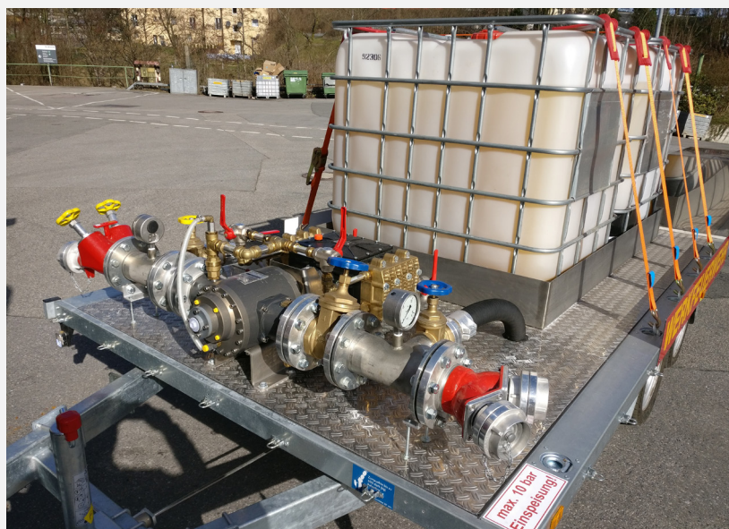
Foam trailer for Hexion GmbH , Germany, with FIREMIKS 2400-1-2-3-4-5-6-PP-F, 2400 lpm and selectable 1-6% dosing rate.
