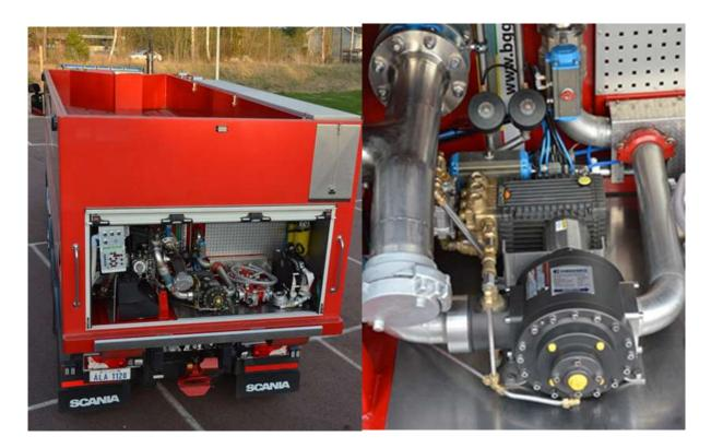
Finland, Åland Island, Jomala Fire Brigade - FIREMIKS 1800-0,3-0,6-1-PP-F mounted on a 24-tonne multi-lift system with two 200-litre foam concentrate tanks and a 15,000 litre water tank, with an additional 7,000 litre open pool on the roof. The unit offers three selectable dosing rates 0,3%, 0,6% and 1% and is intended to be used specifically for the local airport and large-scale fires on the island.
