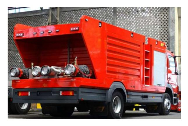
Indonesia, two Foam trucks built by PT Meco Inoxprima for Pertamina, State oil company, each truck equipped with 2 x FIREMIKS 8000-3-GP-F-ALU, giving total 16,000 lpm capacity of dosing 3% concentrate.
