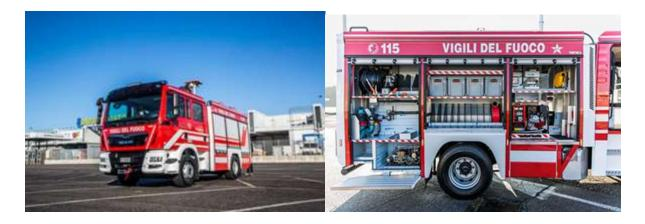
*Italy, Vigili del Fuoco, Lumezzane – Brescia - FIREMIKS 450-1-2-3-PP-M-ALU* installed in a MAN truck, to be used Mobile. Flow range 100-450 lpm and selectable dosing rate 1-2-3%, max pressure 16 bar.
