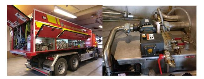
**Sweden, Medelpad Fire Brigade - FIREMIKS 400-1-2-3-PP-F** on a multi-purpose hook-lift system. Flow 100 – 400 lpm, dosing rate selectable 1%, 2% and 3% of X-fog concentrate to be used with handheld nozzles.
